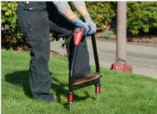
The AF-600-EUR A-Frame pinpoints fault locations with the UAT-600-TE Transmitter
